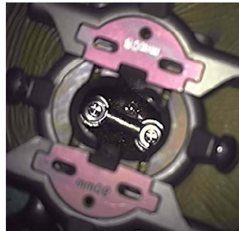
Fig. 30. The set screws are tightened and the extension tabs are removed.
